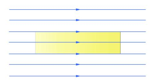
If specimen has no magnetic response, flux lines are not perturbed
