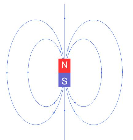
A simple bar magnet behaves like a magnetic dipole
