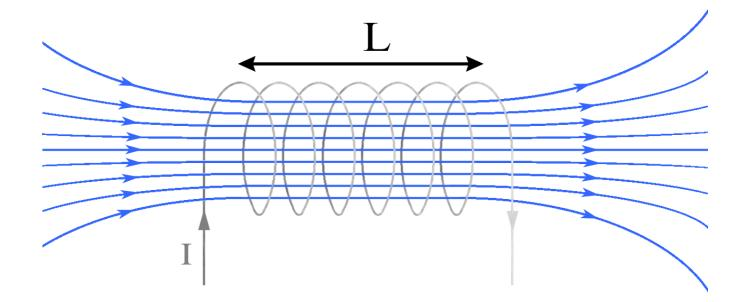
An electric current run through a conducting coil (solenoid) generates a uniform flux density within the coil
