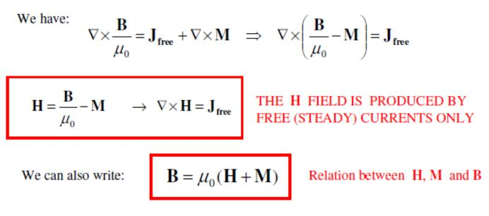
This reveals the components of **B** due to free currents and to magnetisation, i.e. **H** and **M**. Note that **H** and **M** have the same dimensions (A  $m^{-1}$ ).
