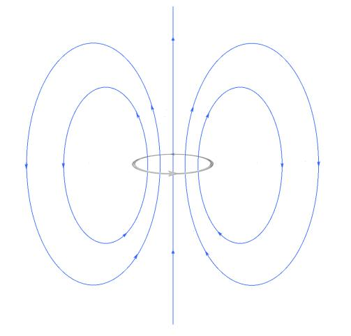
A loop of electric current generates a magnetic dipole field
