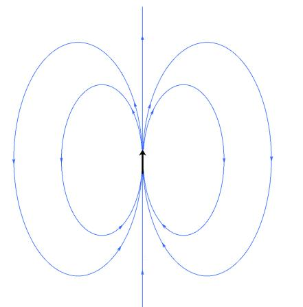
A magnetic dipole is often represented schematically as an arrow.
