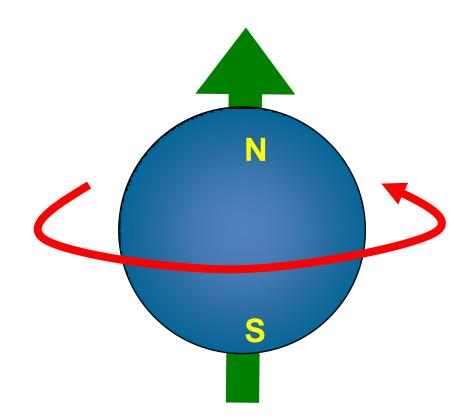
Magnetic fields are generated by movement of electric charges
